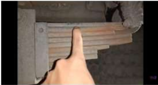
Fig.1. Truck Leaf Springs that have been Added 3 Pieces, Broken Due to Overload.
